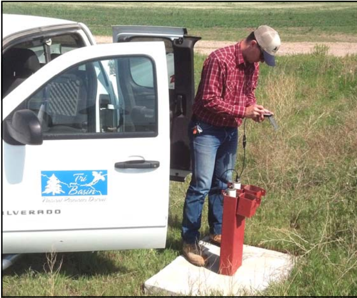
Nolan Little, Tri-Basin NRD Water Resources Manager, measures the spring groundwater level in an observation well in Kearney County.
