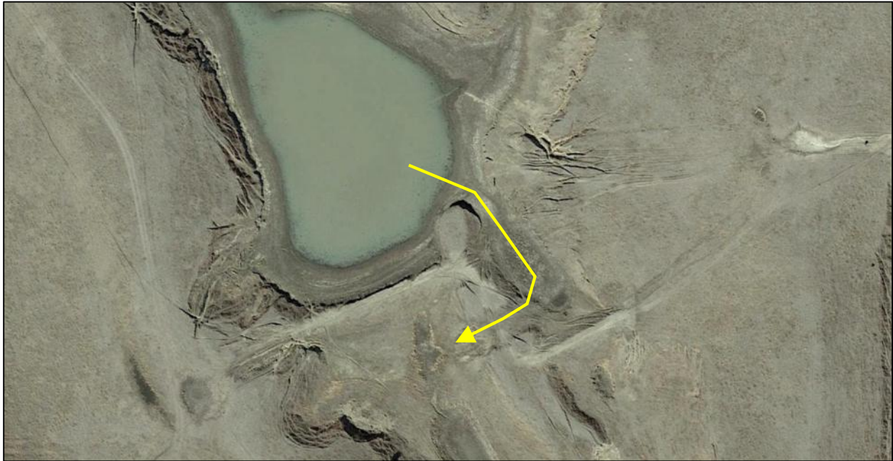
Figure 23. View of pond, dam, and spillway (yellow line) located 1,500 feet upstream of the Farm Road (Rd 738) crossing.
