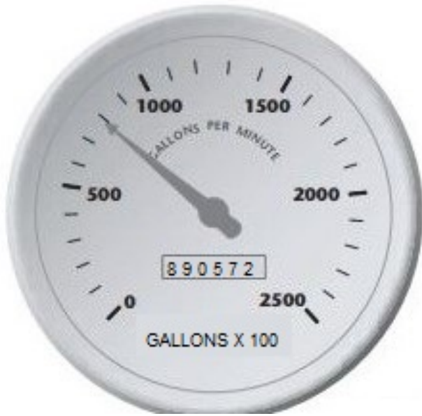
8" Dial Face with Gallon Totalizer x 100 Add 2 zeros to the 6-digit dial face reading. Total Gallons = 89,057,200
