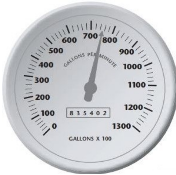
6" Dial Face with Gallon Totalizer x 100 Add 2 zeros to the 6-digit dial face reading. Total Gallons = 83,540,200
