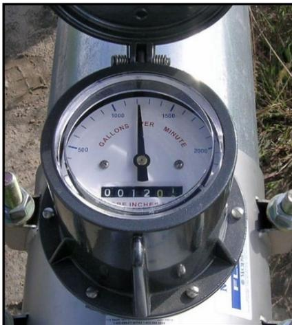
It has also come to our attention that producers who have **Senninger brand flowmeters** may want to make sure the batteries they are using are the correct size. **These meters take lithium 3.6-volt batteries, NOT standard 1.5-volt AA batteries.** Using standard AA batteries will cause these flowmeters to not work properly.
