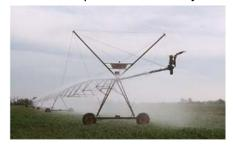
reaches a corner and spew large quantities water. If the field corner is downhill from the outer edge of the pivot, a dump valve can irrigate it, but it doesn't apply water very efficiently. Pivot dealers also sell corner systems that extend out as the pivot reaches a corner and fold back as it moves away. These systems work, but they are expensive, especially in terms of cost per acre irrigated.
