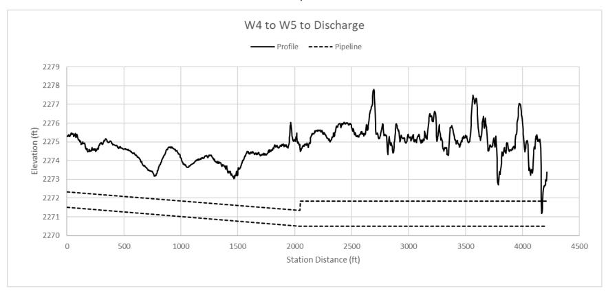
Pipeline alignments with estimated bury depths/elevations. Bury depths and elevations will be finalized with the selected contractor and will be staked by the NRD.
